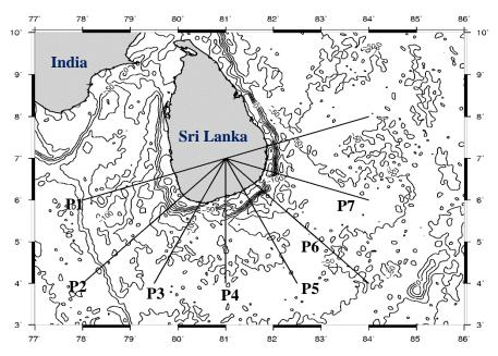
Figure 1. Gravity anomalies over the continental rise of the Sri Lanka (Contours in mGal). Straight lines give the positions of the gravity profiles subjected to interpretation.
