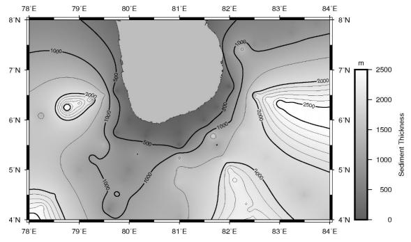
Figure 7. Sediment Thickness map over the continental rise of Sri Lanka based on the gravity study. Contours in intervals of 100 m.
