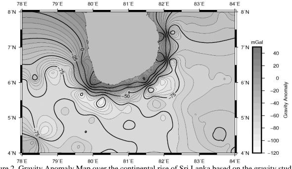
Figure 2. Gravity Anomaly Map over the continental rise of Sri Lanka based on the gravity study (Contours in intervals of 5 mGal).
