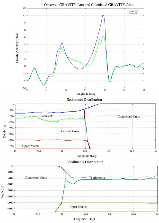
Figure 5. Interpretation of the profile P1 of Figure 1 Contd; (Top: Observed and calculated gravity anomalies; Middle: Left half of the causative body; Bottom: Right half of the causative body).
