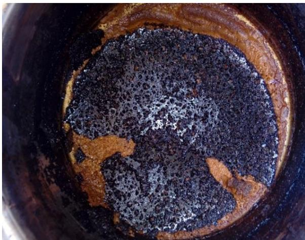
Figure 5. Synthesized modified resin-After the heat treatment.
