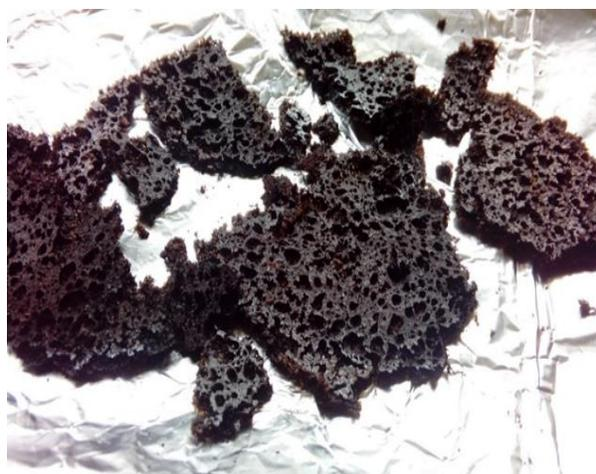
Figure 6. Synthesized modified resin-After the complete removal of oil.
