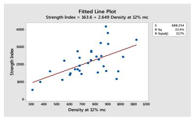
Figure 8. Regression between density and strength index.
