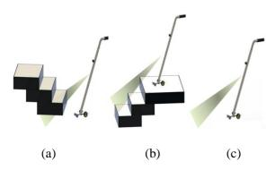
**Figure 2.** Detection of ascending and descending stair obstacles
