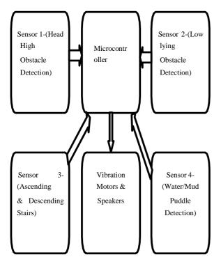
Figure 1. Basic Block Diagram of the design
