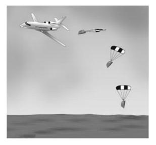
**Figure 3.** Proposed Chute mechanism ought to implement in Deployable Recorders
