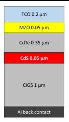
**Figure 1.** Structural view of baseline MZO/CdTe (Top) and CdS/CIGS (Bottom) solar cell (Ehemba et al. 2017).
