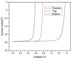
Figure 2. I-V characteristic curves
