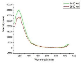
**Figure 6**: Fluorescence results of used engine oil samples.
