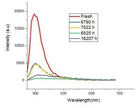
**Figure 3**: Different Fluorescence spectra obtained for Mobil XMP 320 wind turbine gear oil sample
