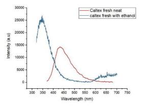
**Figure 7**: Solvent effect of ethanol in engine oils.
