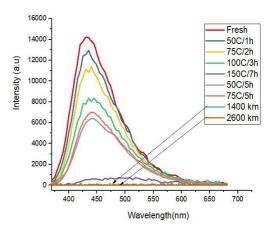
**Figure 4**: Different Fluorescence spectra obtained for artificially aged and literarily aged Caltex DS 40 engine oil samples.
