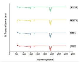
**Figure 2**: Different UV-Visible spectra obtained for Mobil XMP 320 wind turbine gear oil samples.
