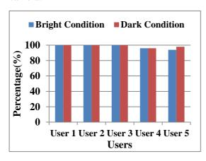
**Figure 6.** Accuracy of office assistant robot system according to the user commands in both bright and dark lighting conditions
