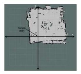
**Figure 3.** The generated local map of the unstructured room used for testing
