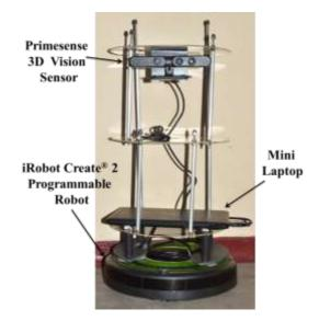
**Figure 1.** Structure of the Office Assistant Robot System
