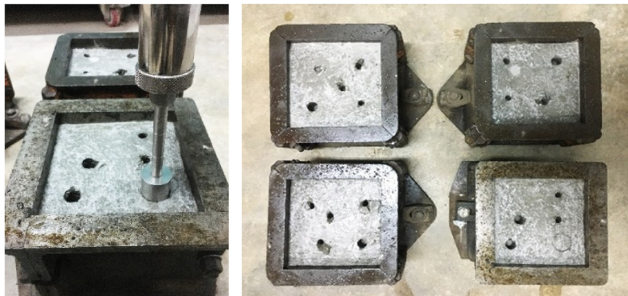
Fig. 4. Penetration of code 1. needle (bearing area of 645 mm 2 ) and specimens for initial setting time test.
