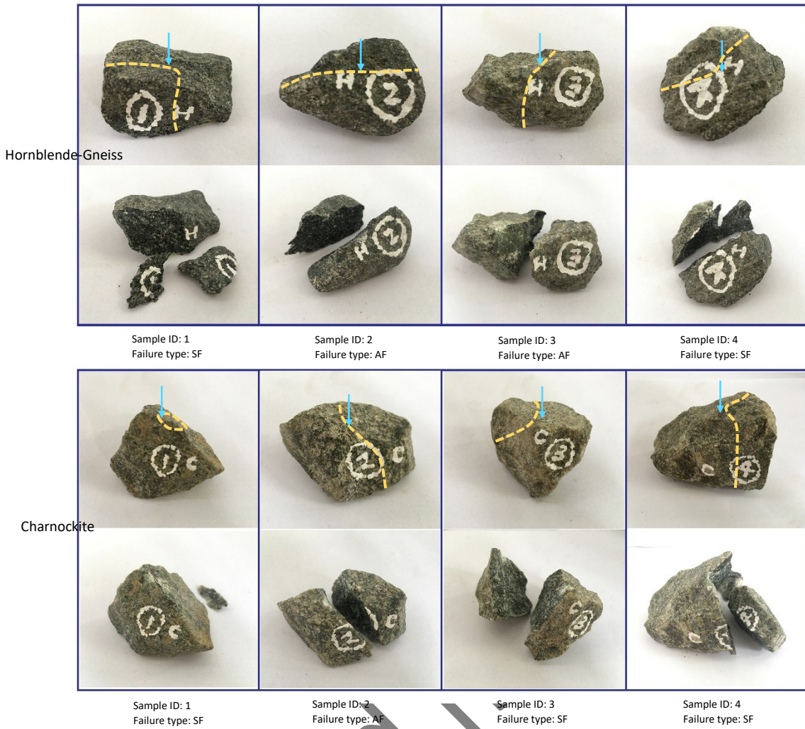
Figure 9. Failure planes of typical rock specimens with respect to load applied (SF: Shear failure; AF: Axial failure)
