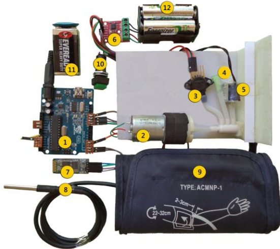
Fig. 7. Device setup of the sensor node. 1 – Arduino uno with atmega328 microcontroller, 2- Air pump (6V), 3- MPX5050 pressure sensor, 4- Small air outlet valve, 5- DC6V Solenoid exhaust valve, 6- L9110 Stepper Motor Driver, 7- HC-06 Bluetooth module, 8- DS18B20 temperature sensor probe, 9- Pressure cuff, 10- power switch for motor drive, 11- 9V Battery and 12- 6V power source.
