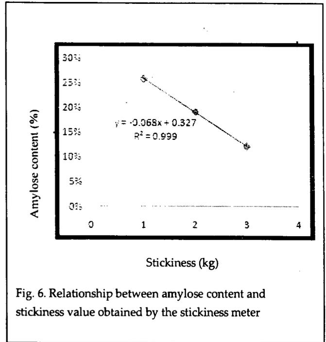
Fig. 6. Relationship between amylose content and stickiness value obtained by the stickiness meter
