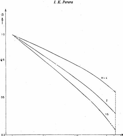
Fig.12. Variation of the parameter ( $\beta$ ) with injected photon denisity  $\phi_2$  for different magnifications.
