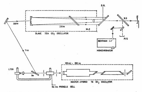
Fig.11. Experimental configuration employed to investigate IML in refs. (35) and (42).
