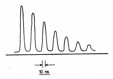
Fig.13. Typical output pulse when injected signal saturates the slave laser gain medium at threshold.
