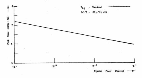
Fig. 6. Energy of the peak power pulse shown as a function of the injected power for a~1 ns pulse.
