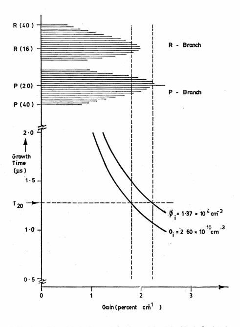
Fig.10. Lower—Gain switched pulse growth time for two injected signal levels,  $\phi i$ , plotted as a function of gain.  $T_{20}$  — growth time of  $P_{10}(20)$  transition from spontaneous emission.
