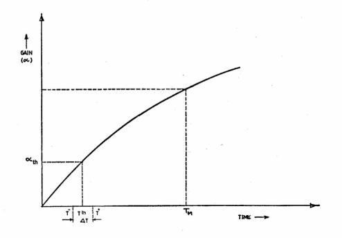
Fig. 1. Small signal gain profile during the time of the laser pulse. T<sup>-</sup> ≤ Time of injection for locking ≤ T+ Time of injection for amplification ≥ TM
