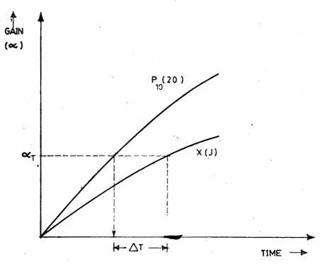
Fig.15. Gain curves of  $10 \mu$  M band CO<sub>2</sub> laser transitions during the growth of the laser pulse.
