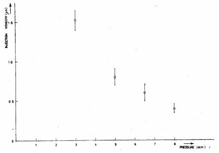
Fig. 8. Variation of injection time window with gas pressure in the slave laser.
