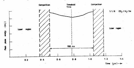
Fig. 4. Characteristics of IML for an injected pulse energy of  $10^{-13}$  J ( $\infty = 1.3\%$  cm<sup>-1</sup>).
