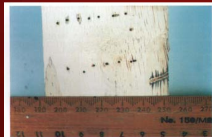
Figure 5.3 Black stained bore holes and tunnels of ambrosia beetle infestation
