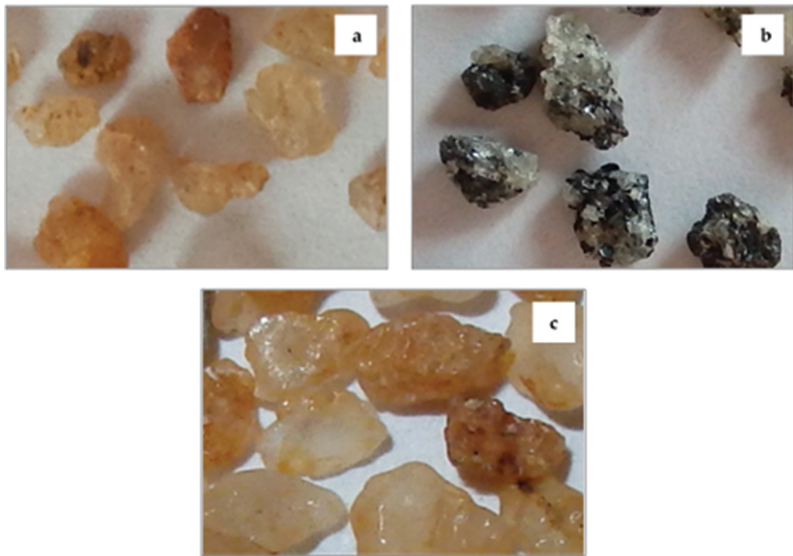
Figure 1. Particle images (size range 1.14–2.28 mm) – (a) river sand; (b) M Sand; (c) offshore sand (Nanayakkara 1999).
